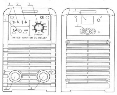
1 Power pilot lamp This pilot lamp when lit indicates that the machine is on.
