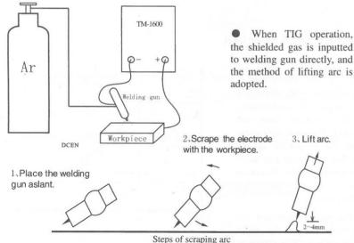
Stricking arc of TIG operation: when tungsten electrode touches the workpiece, the short-circuit current is only 10A. After generating arc, current can rise to the setting welding current. If the tungesten electrode touches the workpiece when welding, the current will drop to 10A within 2s, which can reduce the tungsten spoilage farthestly, prolong the using life of the tungsten electrode, and prevent tungsten clipping.
