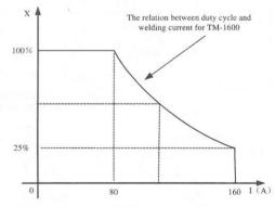
The relation between the duty cycle "X" and the output
